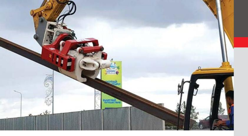
OMS Side Grip Vibro Hammer can handle, pitch and drive the sheet piles. It is capable to accomplish the whole pile driving process without need for manual handling of the piles or assisting machinery.
